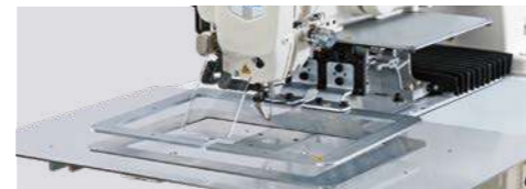
★The picture shows the sewing machine with a separately-driven feeding frame. The separately-driven feeding frame can be selected only for the AMS-210EN/L1306 and AMS-221EN/L2516.
