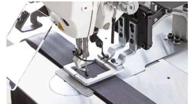
Example application: Reinforcing the stitching of seatbelts *The feeding frame is special order item.
